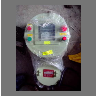
FLP Multi Mill Control Panel
